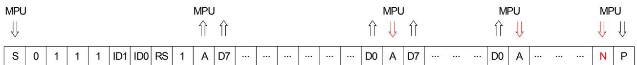
2-wire Serial Interface (I 2 C)-Read mode
